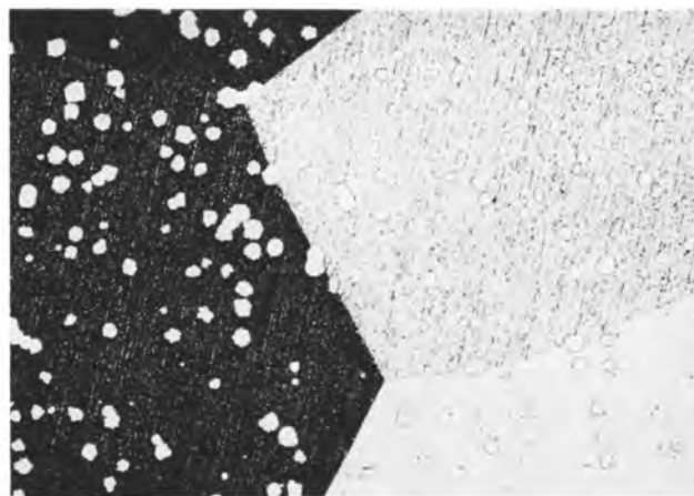
Fig. 3. Photomicrograph of AgMg + \alpha -Ag solid solution, etchant \text{H}_2\text{SO}_4 , \text{CrO}_3 , + \text{H}_2\text{O} . 100X.
