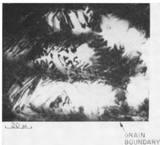
Fig. 6b. Chemical replica of 9½% Sb-Pb alloy showing typical as-cast structure with eutectic segregation continuous at the grain boundaries and interdendritic areas. Light areas are primary Pb dendrites and dark material is segregated Sb.
