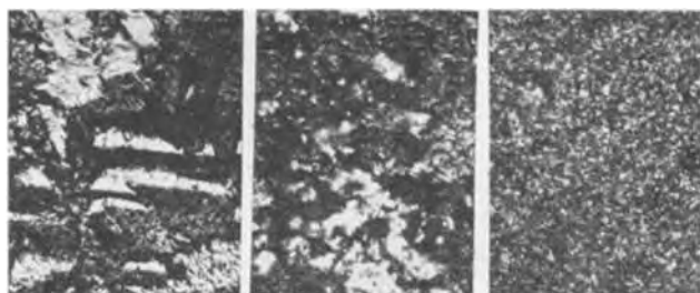
Fig. 1. (Left) Cu base; (center) Pb deposit under conditions of Table I-3, 19 amp/ft 2 ; (right) same with gelatin. Magnification, 500X before reduction for publication.
