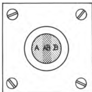
FIG. 2. Top view of the cell. Region A: metal powder alone in castor oil, no luminescence; region B: phosphor powder alone in castor oil, no electroluminescence; region AB: mixture of metal and phosphor powder in castor oil, electroluminescence.
