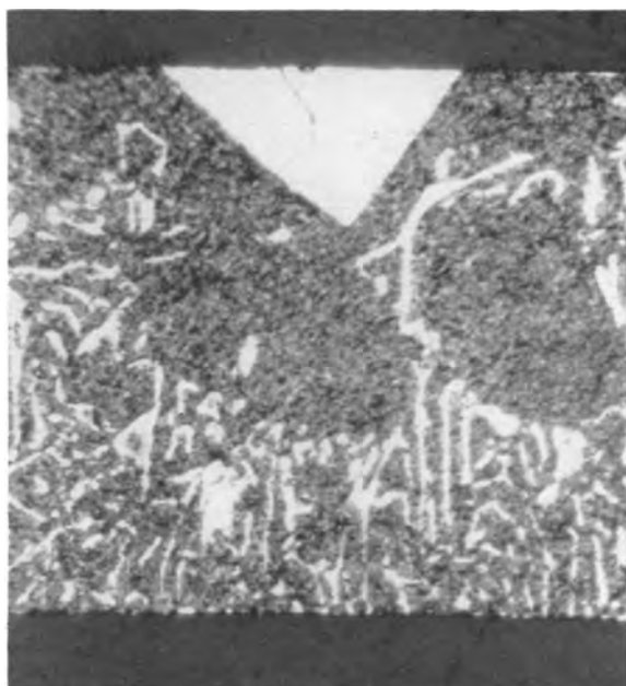
FIG. 7. Cross section through thin Pb-Sb foil. Primary tetrahedral Sb crystal (bright triangle at right edge) is surrounded by an area in which Pb predominates. This dark area isolates the primary crystal and also outlines the shape of the dendritic Pb crystal. Remainder of Sb in picture represents "eutectic" structure formed upon relief of supercooling. 500 \times .
