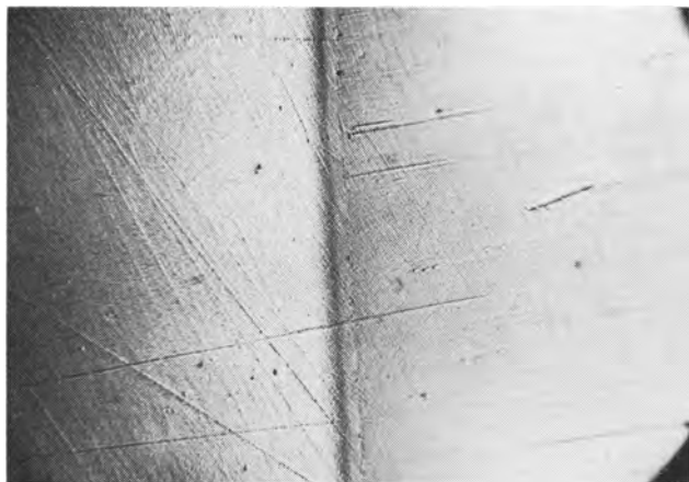
Fig. 3. Part of a metallographic section of a very good filament. The seed is at the left, the deposit at the right. The total width of the picture corresponds to about 0.003 in. (0.075 mm). Most of the apparent imperfections are surface scratches and grain.
