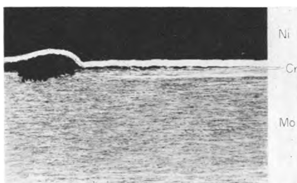
FIG. 8. Cr and Ni on Mo sheet in a zone that blistered when heated. 100 \times before reduction for publication.
