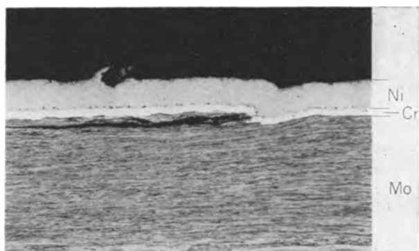
FIG. 7. Cr and Ni on laminated Mo sheet. 250 \times before reduction for publication.
