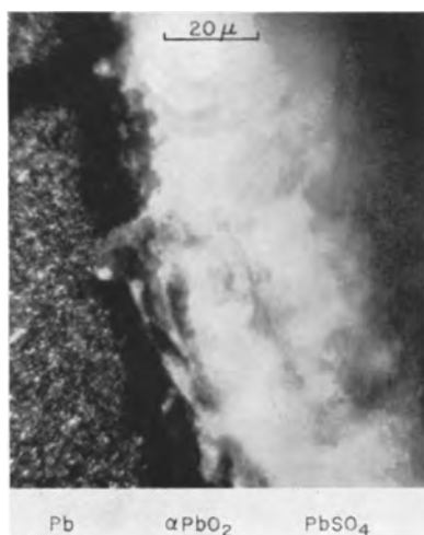
Fig. 8. Plastic mounted section of discharged PbO 2 coating on Pb showing PbSO 4 and heavy layer of αPbO 2 . Magnification 1000x before reduction for publication.
