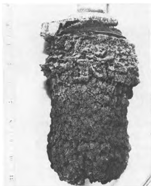
Fig. 2. Typical Th cathode deposit prepared by electrolysis of \text{ThCl}_4 -NaCl system.
