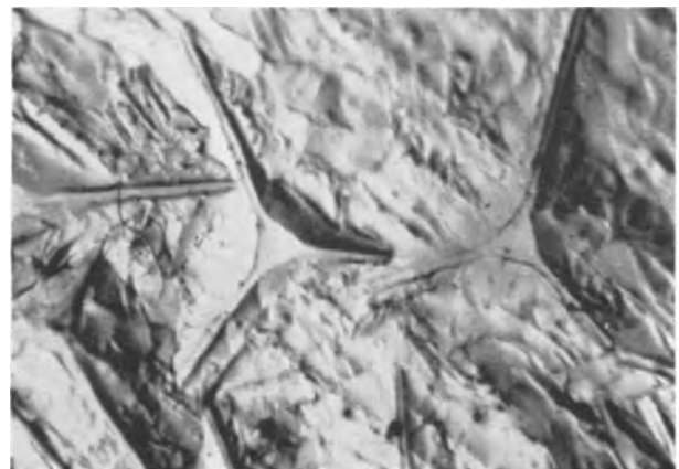
FIG. 2. Primary Sb crystals of primitive dendritic form, crystallized in the as-cast surface layer of a Pb-Sb alloy containing 9% Sb. 800 \times .
