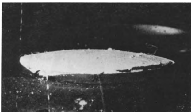
Fig. 4b. Stages in the growth of Cu filaments: after electrolysis for 27 hr.
